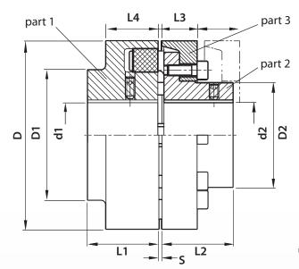
materials: coupling half EN-GJL-250 flexible elements NBR 80° Shore A
